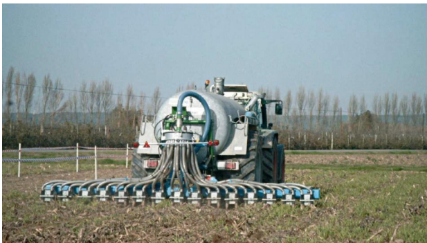
A slurry tank with an injection system.
